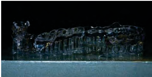
Immediately after the printing process in the ASIGA-Pro2. The splints here are still on the build platform.
