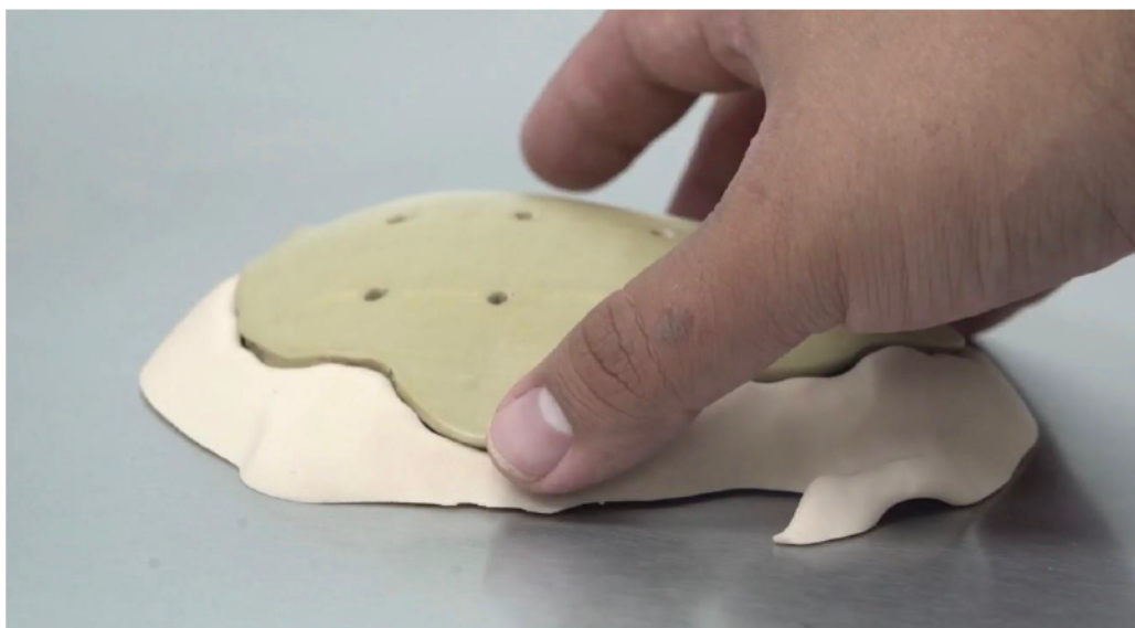
Figure 1. Physical verification model used to evaluate the relationship between the patient-specific cranial anatomy and the proposed reconstruction.
